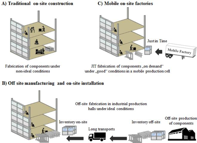
Fig. 2. Concept of mobile On-site Factories
