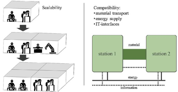
Fig. 4. FR/DP-2: Reconfigurability and scalability of On-site Factories
