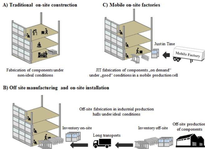
Fig. 2. Concept of mobile On-site Factories
