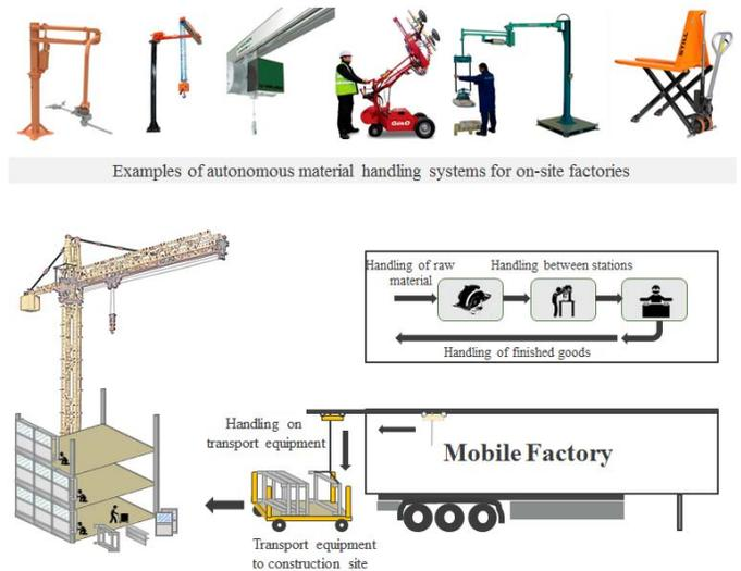
Fig. 6. FR/DP-4: Autonomy in supply and operation of On-site Factories
