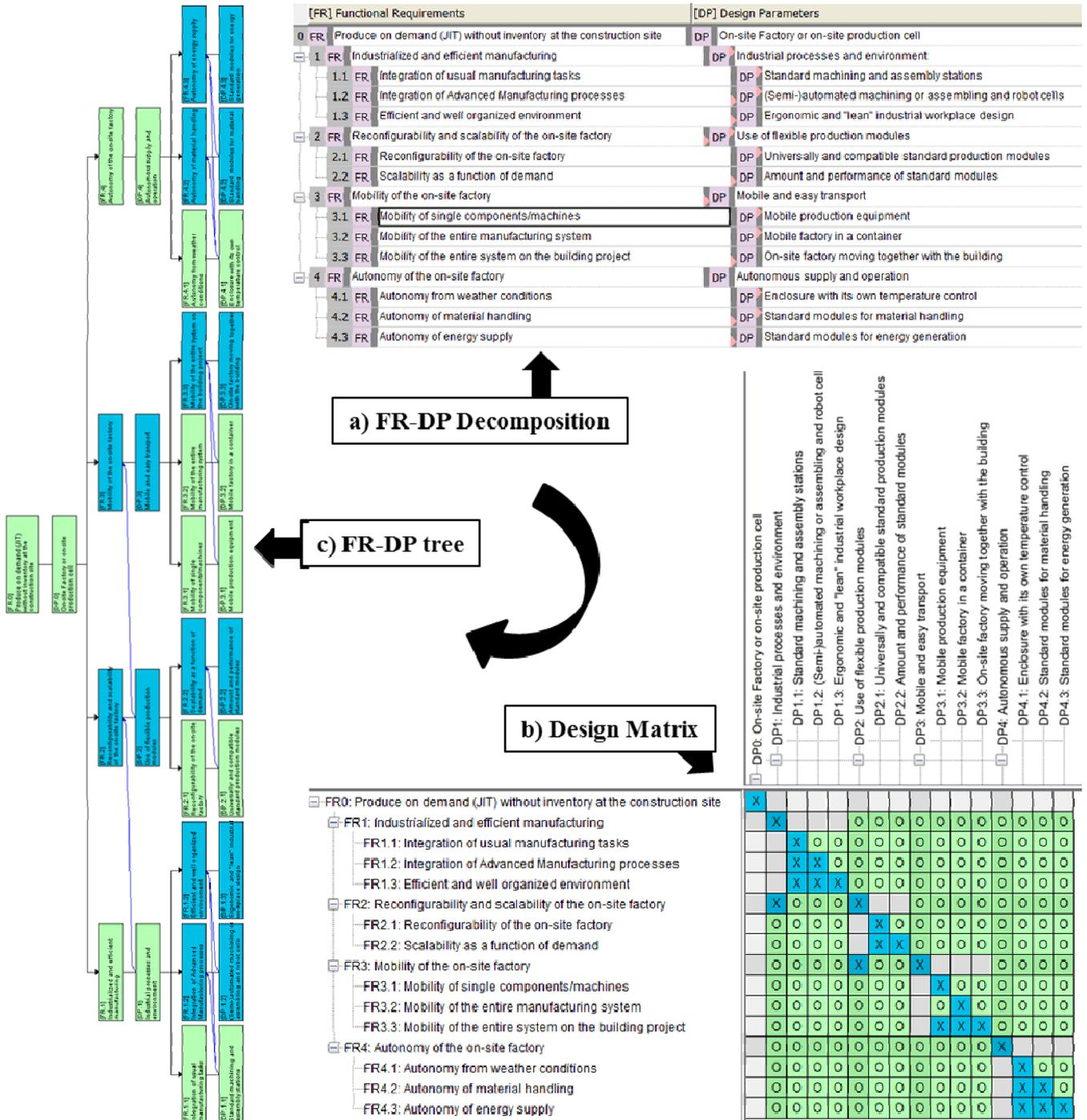
Fig. 7. Axiomatic Design Process for the derivation of Design Parameters in the design of On-site Factories: a) FR/DP Decomposition, b) Design Matrix for the analysis of dependencies between DPs and single FRs, c) Top-down visualization of Design Parameters in the FR-DP-tree (used software: Acclaro DFSS)
